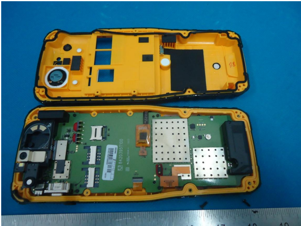
Open view of IPX8 test
