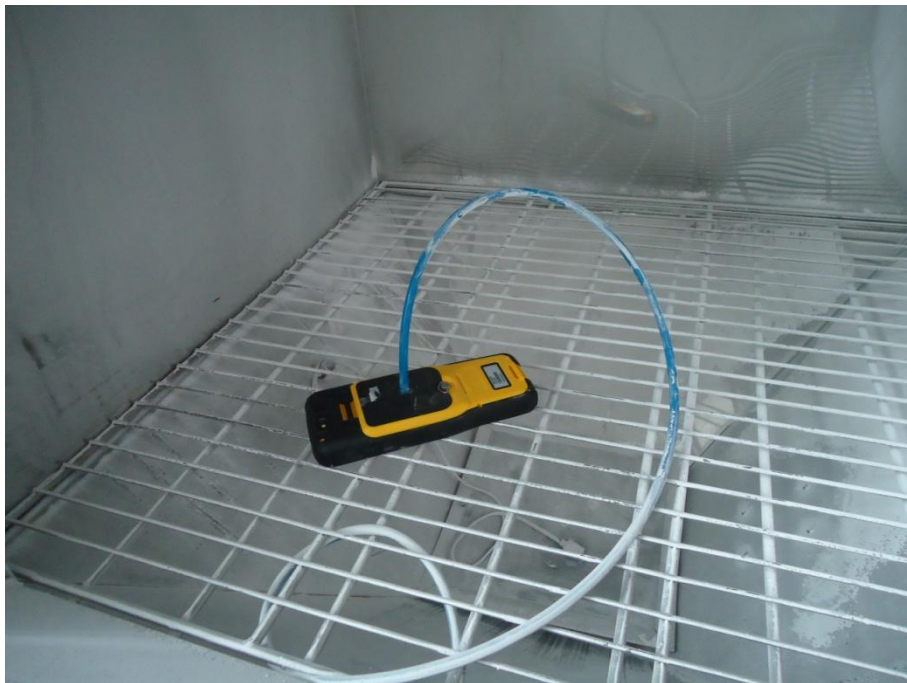
General view of IP6X test
